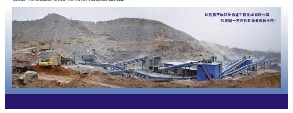
DSMAC advanced sandstone production line includes vibrating feeder, high-performance jaw crusher, high efficiency stone crusher and high abrasion resistance spare parts. The production line has proprietary intellectual property rights and some unique features as follow:
